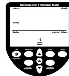
**Projected distance** is the distance projected for the set duration given the current intensity. Projected distance must be selected immediately prior to the workout and is current only for that workout.
