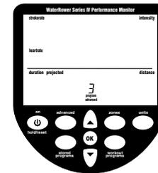
**Projected duration** is the duration projected for the set distance given the current intensity. Projected duration must be selected immediately prior to the workout and is current only for that workout.
