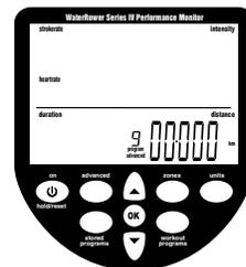
This program allows you to view the Firmware Version (the version of the software that runs the monitor) and the total distance the machine has traveled.
