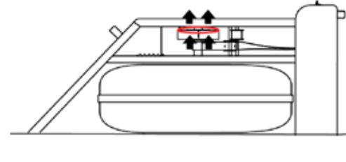
**Solution 2:** Loosen and retighten the bolts on the upper deck and forward riser. If these bolts are not uniformly tightened during assembly, the alignment may be off.
