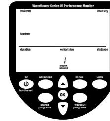
This program allows manual storage of workout settings. This is useful if the S4 monitor is used by numerous users and the AutoStore programs are overwritten.
