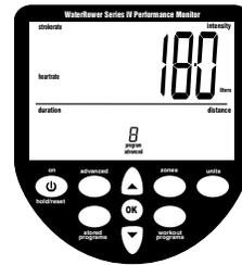
This program allows you to input the volume of water in the tank. The tank volume is necessary in calculation of power (watts).
