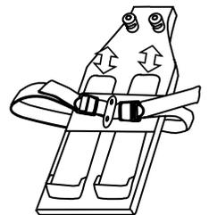
Note: Do not tighten footboard assembly bolts
