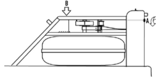
2. **Loosening bolts** - over time and with use bolts can come loose. Use the 5mm Allen key to gently tighten the bolts. If the bolts continue to loosen use a small amount of medium strength Loctite® to fasten the nuts and bolts more securely.
