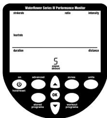
Advanced Program 5 allows you to view the ratio between the power and recovery parts of the stroke. The recovery ratio must be selected immediately prior to the workout and is current only for that workout.
